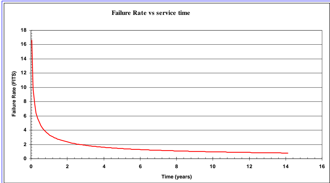
Figure 1. Field failure rate of a component that passed a qualification test for max 40 fits
